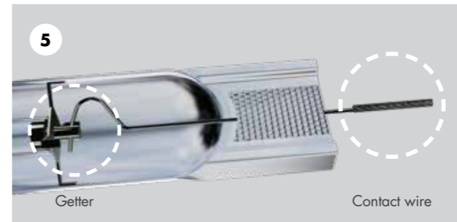
5 Before placing the new lamp, make sure the contact wire is straight, the getter is on the ballast side, and the text on the lamp is facing out.
