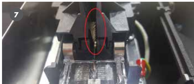
Make sure the contact wire from the lamp is straight between the contact plates inside the fitting
