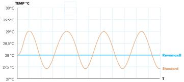
Stable output (supply) temperature, during dehumidification at night or day with the Pro4 the output temperature can go up as high as 40°C and as low as 10°C depending on the indoor temperature during dehumidification.
